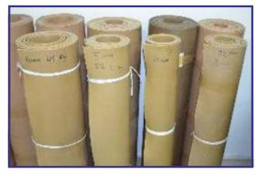
For surface coating in sandblasting rooms a soft, high-strength material. It also creates vibration and noise. It can be used safely under the machine.
