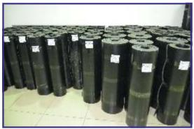
Nitrile plate has very good resistance to gasoline and petrol. It withstands pressure of 200 kg/cm2 with normal formulation. It can elongate 370%. to friction
