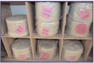
Synthetic additive cotton yarn with paraffin and special oils. square section with 2-3 layers of diagonal mesh impregnated as manufactured. In ship shafts, cold water engines, pipe connection sockets, It is used for sealing in shaft slots.
