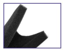
In central type ventilation systems, pre-filter in fan-coil suctions and split air conditioners used as. Porous polyurethane
