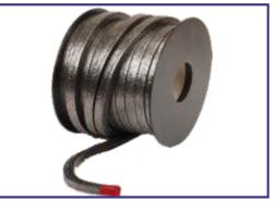
It is made of pure expanded graphite on a linen center. Thermal and chemical resistance, self-lubricating and good Thanks to its thermal conductivity, expanded graphite knitting used in rotodynamic pumps and joints seals are used.
