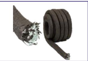
Glass fiber packing then graphite coating being processed. Graphite coating friction glass fiber seal static seal widely used in applications. containers, heat in systems such as heaters, manhole covers and pipes It has insulation and fire prevention properties. Water, steam, air, oil and similar chemical properties It is a suitable material for neutral environments.
