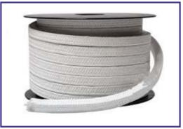
In the knitting process, the knot is impregnated with a special PTFE-based mixture. knitted packing made of natural linen, double function of impregnation exists; It increases the chemical resistance while reducing the coefficient of friction. At the same time, delicate flax fibers are produced and the seal is exceptional. It ensures that it is soft and fits well in the stuffing box.
